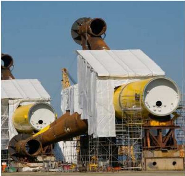
Tripods being welded
