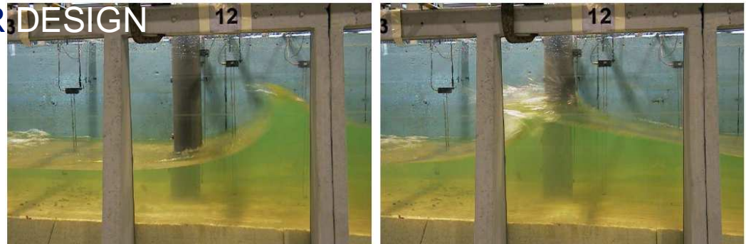
Test EOL59 : bottom slope 5% - d_{\text{offshore}} = 0.8 \text{ m} - T = 2.4 \text{ s} - H_{\text{offshore}} = 0.288 \text{ m}
